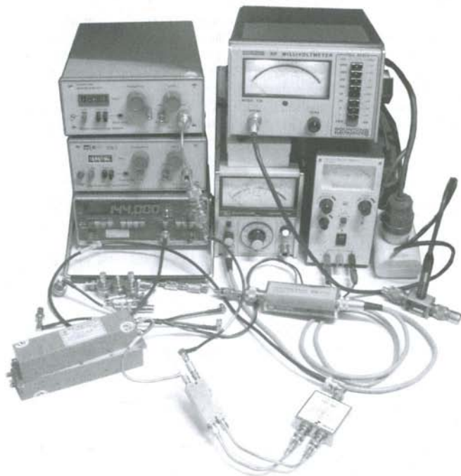
Fig. 3 Setup including a Zeta Labs mod. 4702-01 local oscillator at 9.990 GHz
