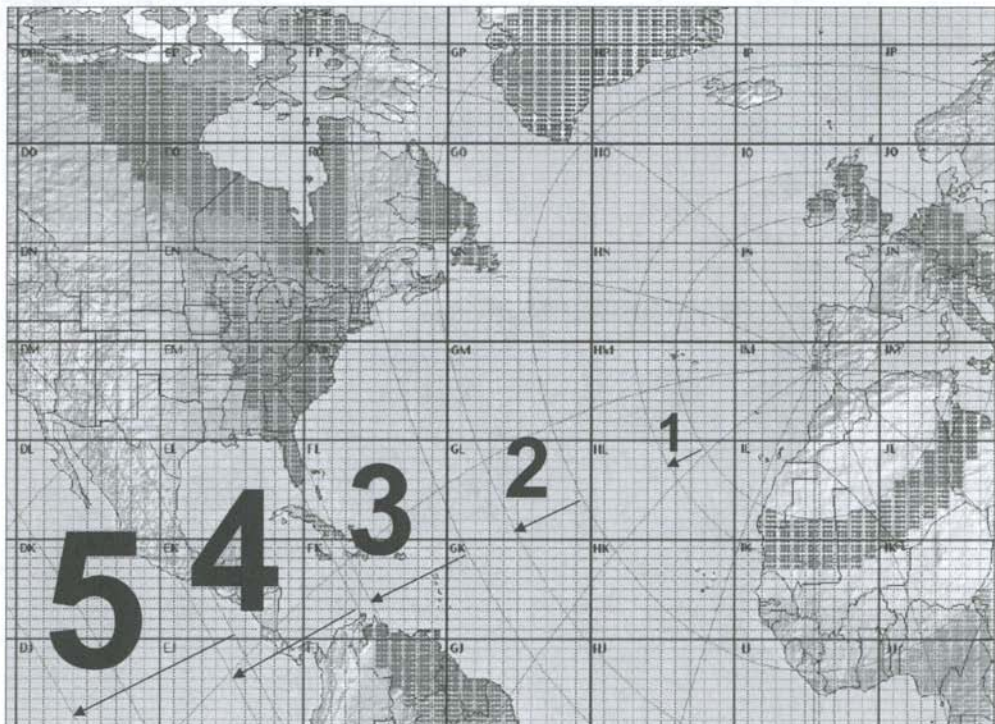
Fig. 7 Simulation of the hop target ranges and areas with the Beamfinder software (by DF5AI) assuming a constant height of 105 km for the E layer. For better illustration a minimum hop distance of 1700km and a maximum of only 2200km was set.
