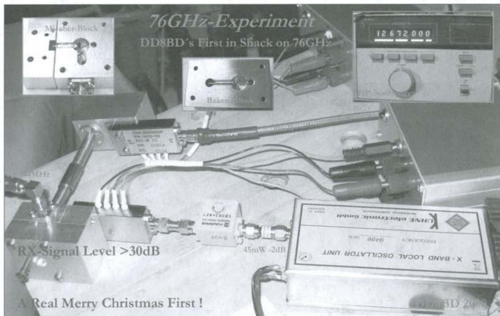
Fig. 9 Complete assembly during the first successful 76 GHz reception
