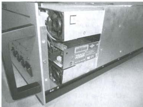
Left: On top and bottom the two 1500 VA switch mode power supply units, in the middle another small switch mode power supply. Right: 4 cables for the double 50 VDC RF-module power supply
