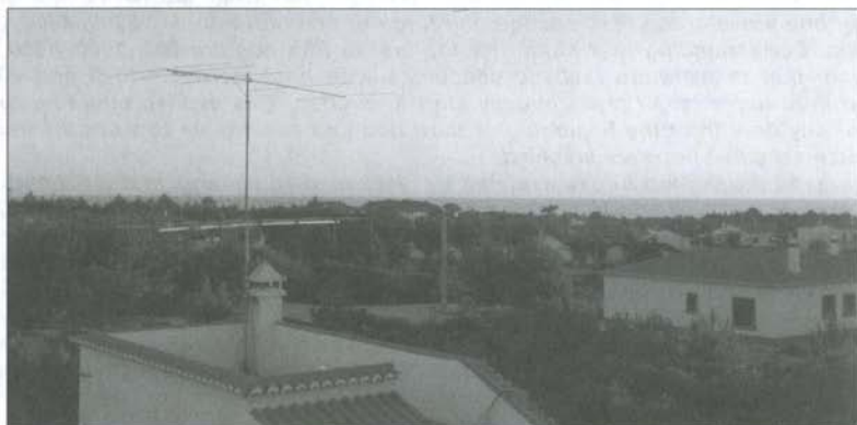
Fig. 9 CT1HZE's takeoff to the U.S. over the Atlantic Ocean with 5 element M2 Yagi for 6m
