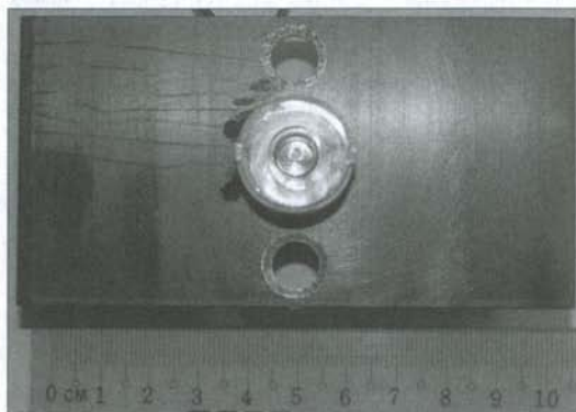
Figure 12: Luxeon with torch lens mounted on Heat sink 14 . Note oversized and chamfered mounting holes which allow adjustment for alignment.
