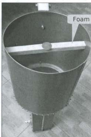
Fig.: A metal coin in the horn aperture enables >60 dB isolation
