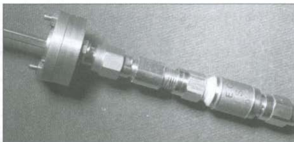
Fig. 3 Adapter fitted to APC connector saver and detector
